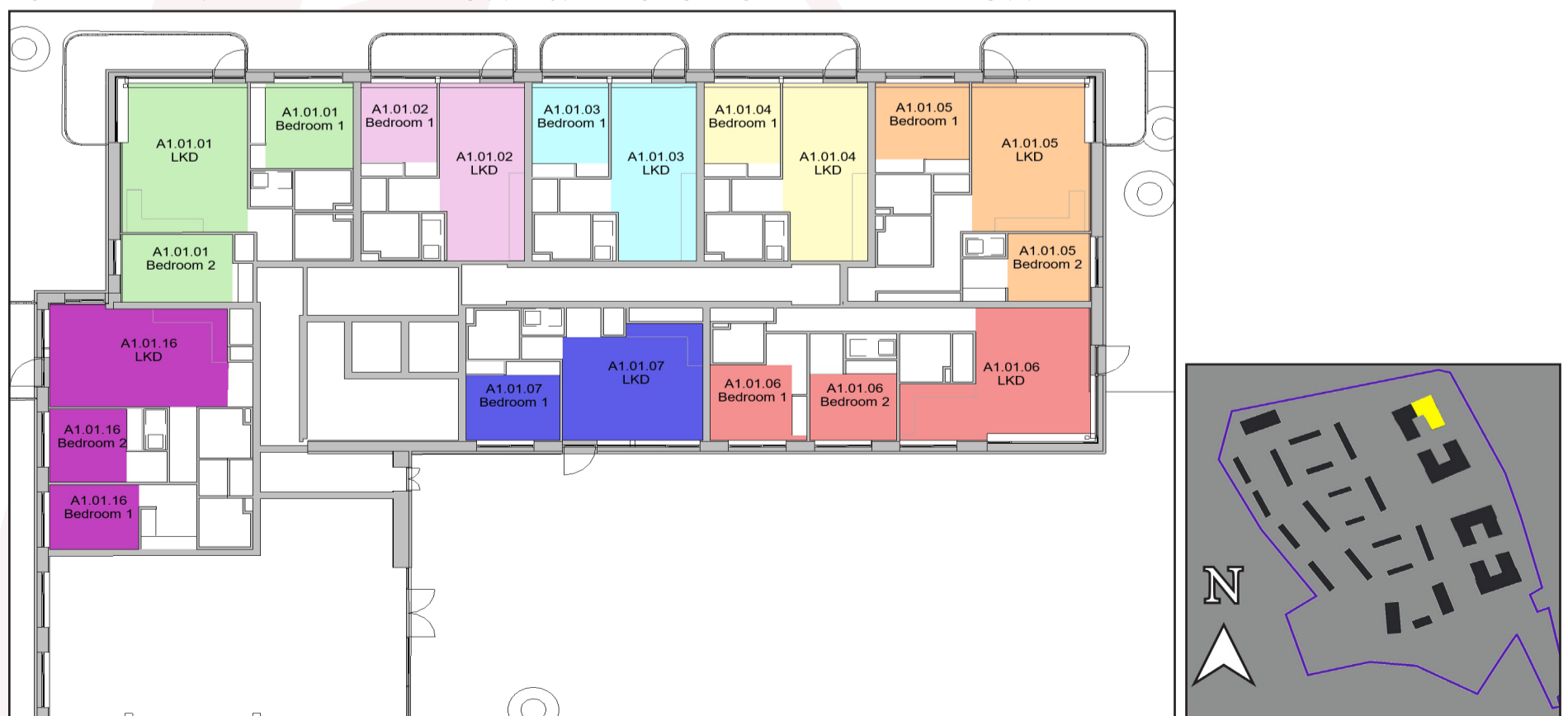
Figure 7.70: Floor plan of assessed building (L), Keyplan highlighting the assessed building (R).
